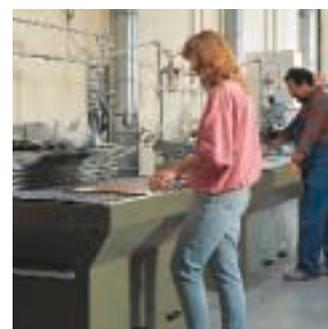
Work protection benches with integrated filter unit are an ideal and inexpensive answer to open machining of different workpieces.
