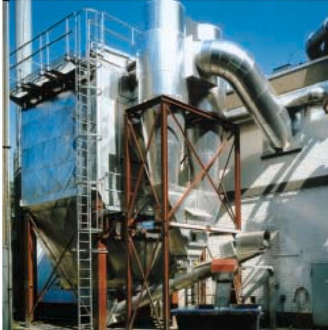
Filters with integrated cyclone pre-separators have proved particularly successful in dealing with large amounts of chips resulting from planing and sawing plants. The useful life of the filter bags is considerably increased, the energy costs for compressed or reverse air reduced to an absolute minimum.
