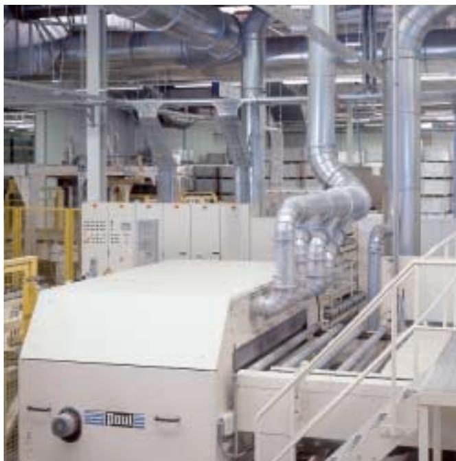
Together with our clients we develop special solutions. Dust is generally removed from the suction points of a machining centre through individual flexible hoses. In the machining centre shown this was not possible because of the low workshop ceiling. A special swivel device was developed so as to overcome the long distance to be travelled in X and Y axis.
