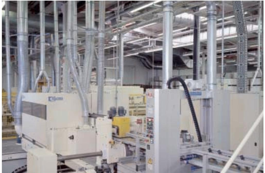
Venti plants can deal with over 100 suction points. Collected dust and chips are carried to the filter system and the following heat recovery plant via a main duct. Air volumes of over 300,000 m<sup>3</sup>/h can be exchanged in this way.
