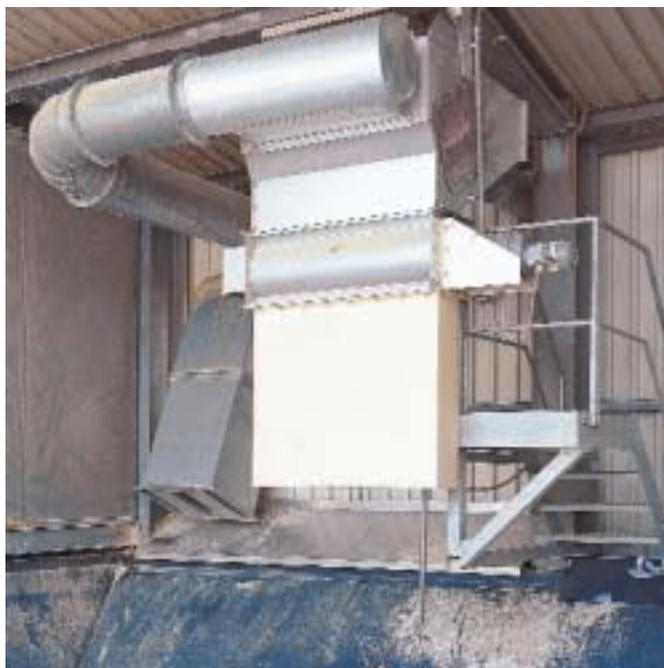
Material separators to remove pieces of material from the air-stream, such as lumps, sawn off pieces, veneer strips, are also included in our manufacturing program.
